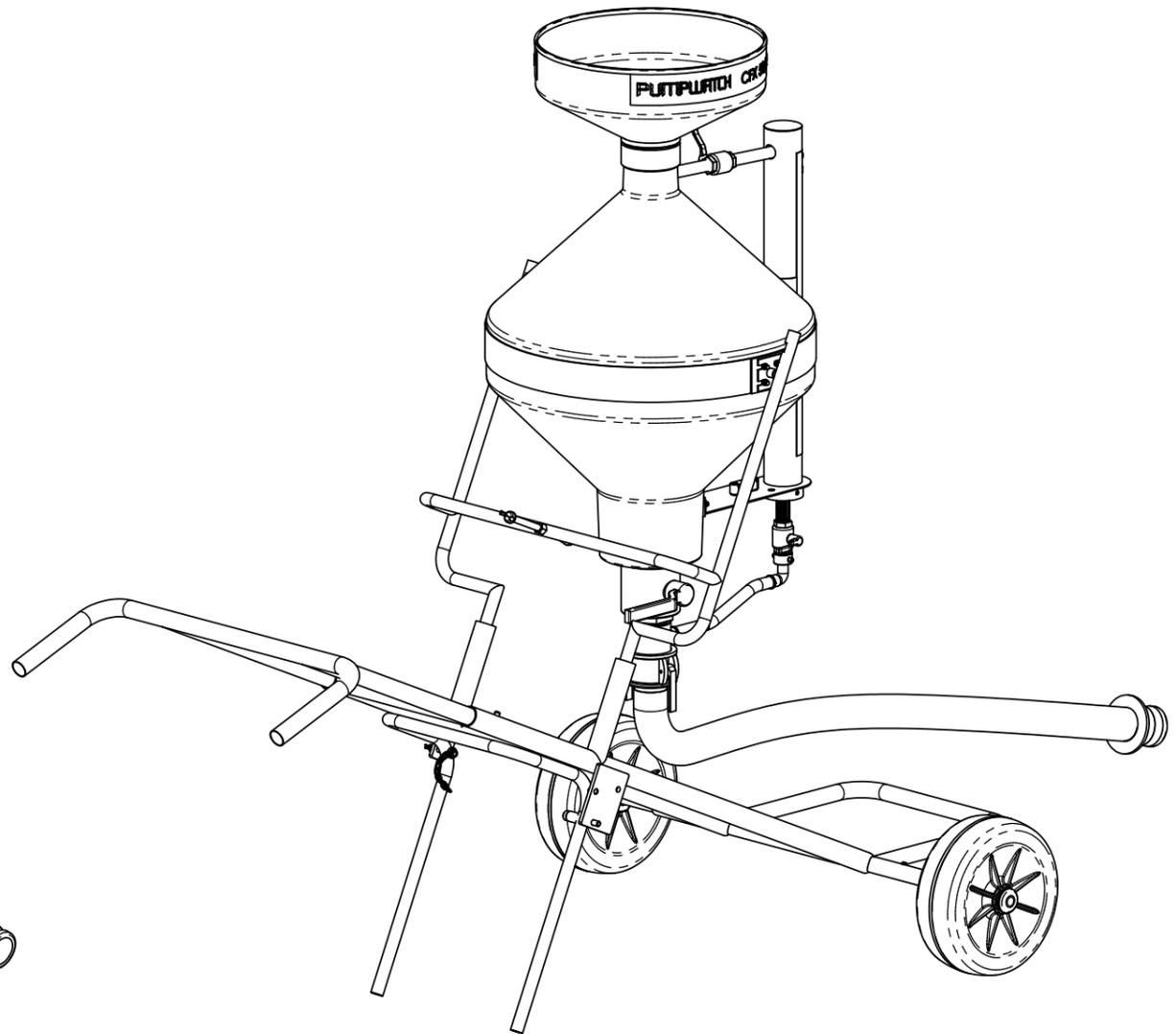
MAIN MEASURE ASSEMBLY COMPLETE WITH SCREW-ON FUNNEL AND QUICK-COUPLING DISCHARGE HOSE, IS SHOWN SUSPENDED FROM A COLLAPSIBLE TUBULAR STEEL TROLLEY ASSEMBLY WITH THE ADJUSTABLE LEG SUB-ASSEMBLY SET IN THE UPPER DISCHARGE POSITION, READY TO DISCHARGE FUEL.
