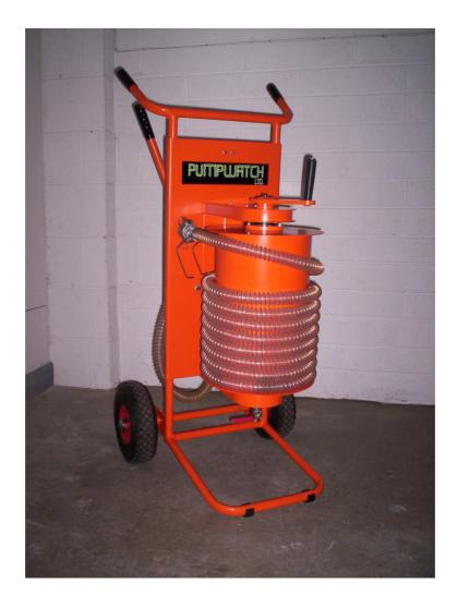
A simple, hand-pumped system to return fuel to over-ground storage tanks or, to return fuel to otherwise difficult to access fuel storage systems.
