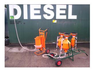
Can be used to connect to any PUMPWATCH Measure Pack discharge hose or siphon most of the fuel from traditional self standing measures
