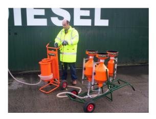
The Hi Return Pump is used in an upright position that allows the operator to stand straight to the pump and maximise its capacity. The contents of a 3-measure Multi Measure Pack as above (45L) are returned to storage in just 3 minutes!
